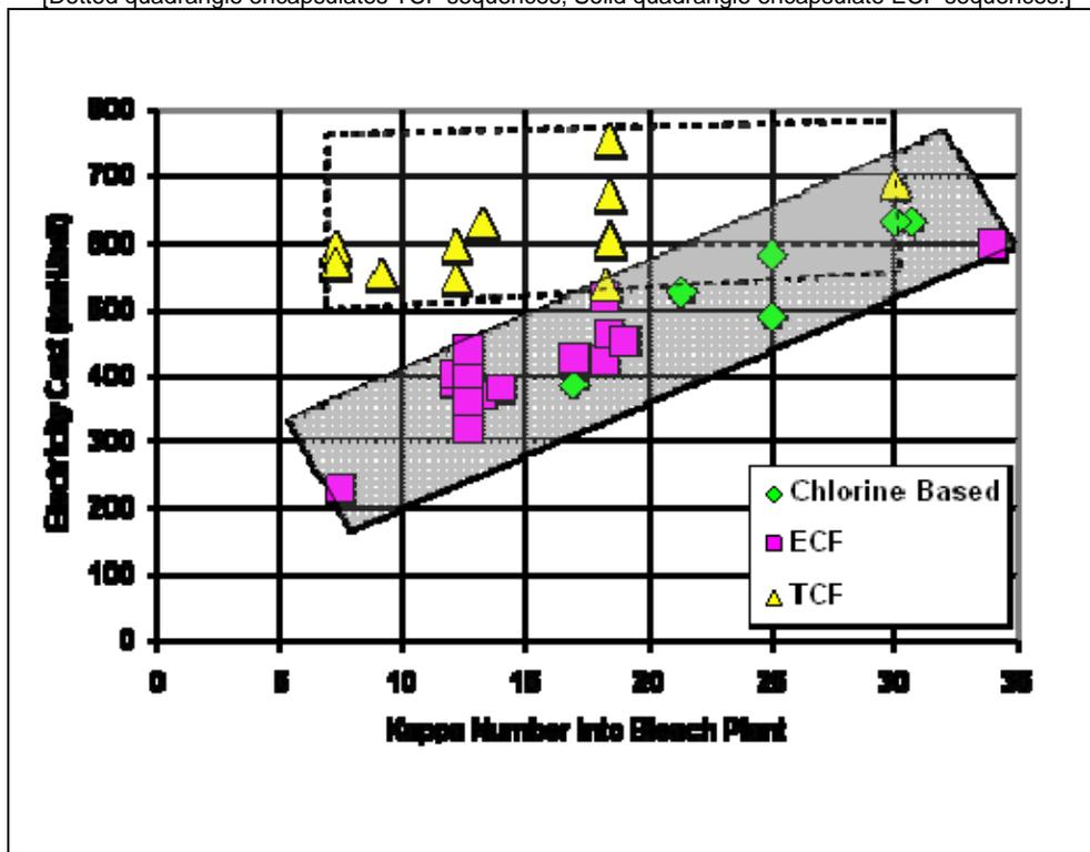
Figure C12. Electrical Energy Requirements for Bleaching Sequences When Including Electricity Required for Stage Pumping and Mixing and Using Higher Electricity Values for  $O_3$  and  $H_2O_2$
