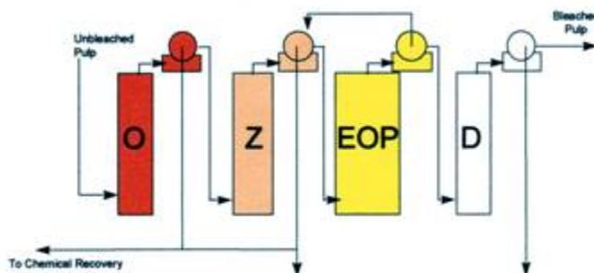
**Figure C18. Bleaching Sequence Showing Alkaline Filtrate Recovery**
