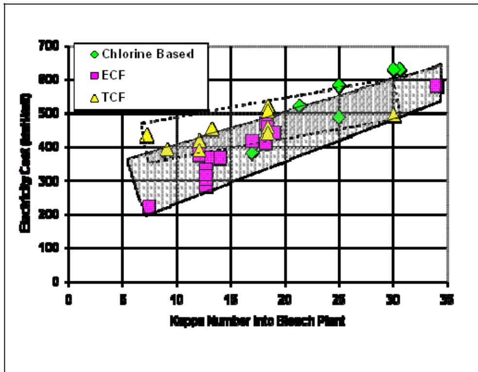
Figure C10. Electrical Energy Requirements for Bleaching Sequences When Including Electricity Required for Stage Pumping and Mixing and Using Lower Electricity Values for  $O_3$  and  $H_2O_2$
