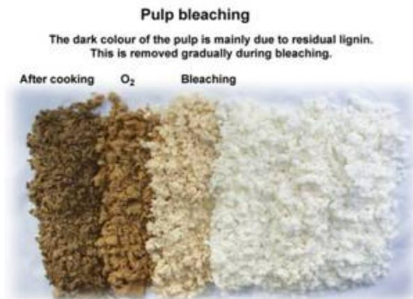
**Figure C5. Illustration Showing the Degree of Color Removal during Pulp Bleaching**
