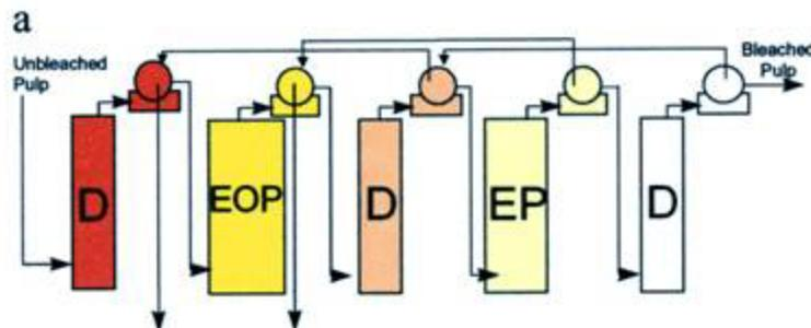
Figure C6. Typical Elemental Chlorine Free Bleaching Sequence
