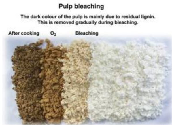
Figure C5. Illustration Showing the Degree of Color Removal during Pulp Bleaching ( http://www.chmltech.com/pulppaper_files/pulp%20bleaching.jpg )
